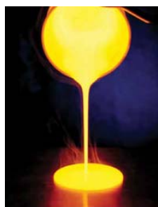
VITRIFICATION Pouring glass to immobilize radioactive waste.
