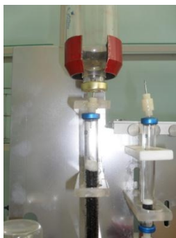
Fig. 17 Ag/C column or AgC/ZrO/AC combination column
