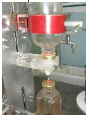
Fig. 15 Pass the sol. through 0.2μm filter
