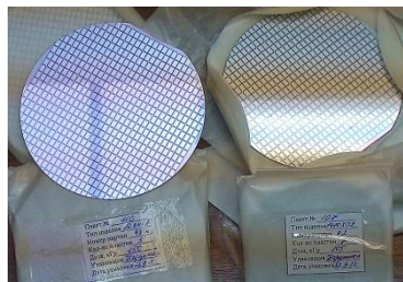
Fig. Silicon semi-conductor plates with preparations of devices after electron beam processing
